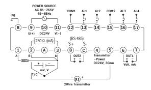
\* mA Input(+ -) Needs 250 OHM 0.05% 25ppm Resistance (2, 3 Pin)
